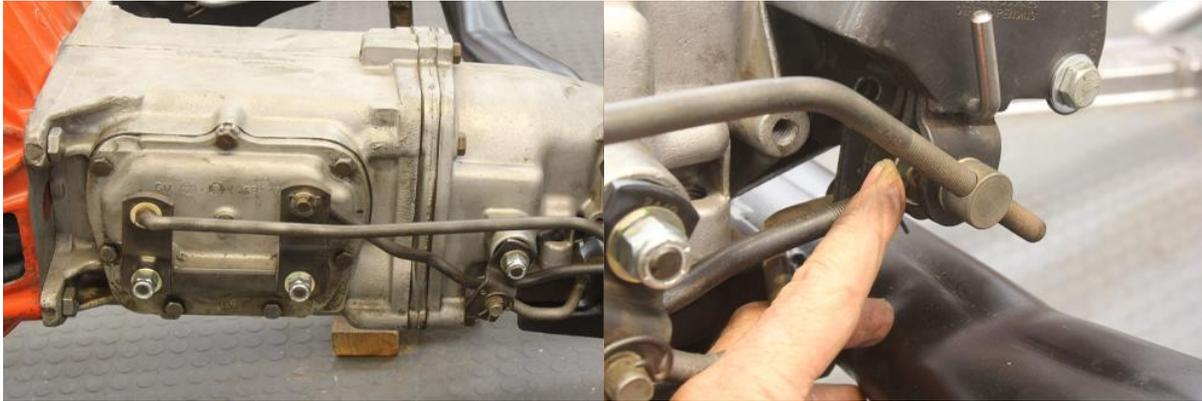
Note how the 3-4 arm angles away from the transmission case and the rod fits through with the pin pointing toward the trans. Adjust the length of the rod and then install the pin into the shifter arm and affix the spring clip.
