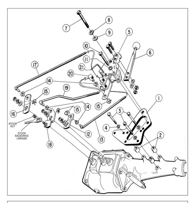
**NOTE:** There are three hole patterns in the mounting plate ( # 1). Use the hole pattern that matches the mounting bosses on your transmission extension housing. If the hole pattern on your extension housing permits installing of the plate in more than one location, use the one that places the shifter stick in the most comfortable position.
