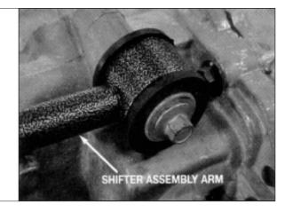
STEP 10. Remove the two (2) hex nuts that secure the rear mount of the shifter assembly to the floor and set aside.
