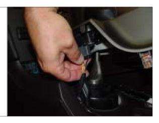
**STEP 5.** Remove rubber dust boot from shift stick by pulling up and out of the floor pan opening and sliding it over the shift stick. Set boot aside.
