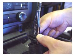
**STEP 25.** Replace the shifter boot that was removed in STEP 2.
