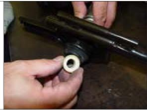
**STEP 15.** Place the HURST shifter on a workbench and insert the two (2) metal flanged sleeves into the bushings in the HURST shifter assembly arm.
