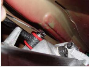
STEP 19. Attach the metal bracket to the rear urethane mount on the HURST shifter assembly and align the holes in the bracket with the two (2) threaded studs on the vehicle. Replace the two (2) hex nuts removed in STEP 10 and tighten securely.
