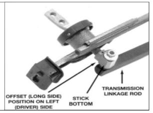
**STEP 21.** Carefully lower vehicle. From inside the vehicle, attach the HURST upper stick to the lower stick with two (2) stick mounting washers and two (2) stick mounting screws and tighten.
