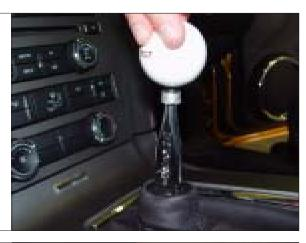
**STEP 33.** With one hand holding the knob in the correct orientation, use the other hand to tighten the knob nut up against the knob.
