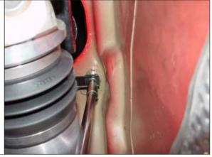
**STEP 11.** Remove metal bracket from the rear rubber mount and set aside.
