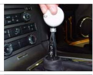
**STEP 33.** With one hand holding the knob in the correct orientation, use the other hand to tighten the knob nut up against the knob.
