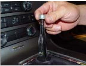
**STEP 32.** Screw on the HURST knob all the way down until it contacts the knob nut, then back it off until the orientation of the shift pattern/logo is correct.
