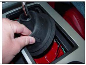
**STEP 24.** Push the rubber boot support onto the HURST chrome stick
