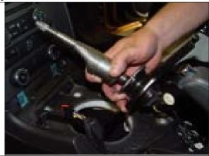
**STEP 13.** Place the factory shifter on a workbench and remove the two (2) metal flanged sleeves from the front rubber bushings on the shifter assembly arm.
