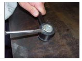
**STEP 14.** Remove the two (2) plastic bushings from the bottom of the shifter. These bushings should be removed by hand to not damage them.
