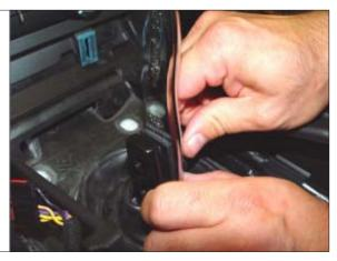
STEP 23. Reinstall the rubber boot that was removed in STEP 5. Push down the lower lip of the boot through the vehicle's tunnel to ensure a proper seal. With the boot in place, test shifter operation. Move shifter through all gears and make sure that it engages each gear fully and that the stick moves freely from side to side in the Neutral position. The knob may be temporary installed to aid in testing.
