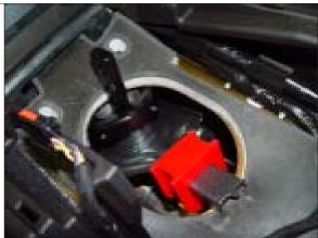
step 18. From underneath the vehicle, work the HURST shifter assembly forward so that the tail end can go through the tunnel opening. (Follow guidelines given in STEP 12). Then attach the front shifter arm to the transmission and insert the hex bolt removed in STEP 9 but do not tighten at this time.
